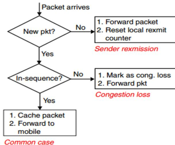
Figure 6: Operation of snoop protocol
