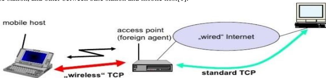
Figure 5: Split connection approach in I-TCP
